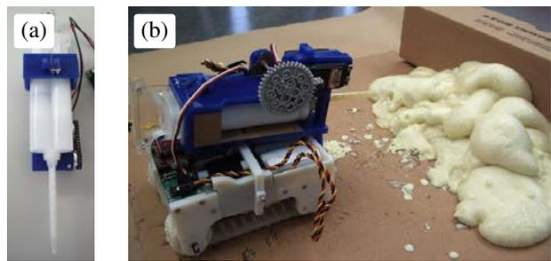
Fig. 5. (a) Bottom view of syringe dispenser for casting foam. The two compartments are actuated by the same plunger and both feed into a single static mixing nozzle. (b) Dispenser mounted on a small remote controlled robot. Cured previous depositions are shown right.
