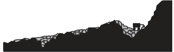
Fig. 1. Diagram of mobile robot building a large ramp in unstructured terrain using amorphous materials. The robot starts on the left and is trying to reach the right. It builds ramps over features it cannot climb using an amorphous material (gray) that conforms to arbitrary obstacles.
