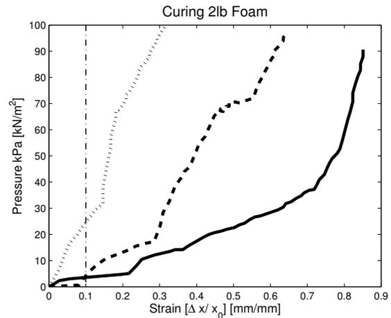
Fig. 9. Stress-strain curve of foam at different stages of curing. The solid line is 20 min after mixing, the dashed line after 25 min, and the dotted line after 30 min. After 20 min the foam is still very soft and compresses almost completely.
