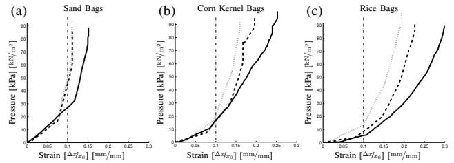
Fig. 8. Stress-strain curve of bag structures. We loosely built a pyramid of 14, ( $3 \times 3$ ), and compressed them repeatedly. In all plots, the solid black line is the first cycle, the dashed the second, and the dotted line the third. (a) Bags filled with sand. Sand bags had the most compressive strength and displayed the most consistent compression behavior for repeated loading. (b) Bags filled with dried corn kernels. (c) Bags filled with dried rice.
