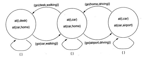
Figure 7.1 Part of the transition system describing the airport domain
