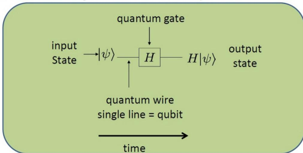
Quantum circuits are sequences of instructions. Describes a series of unitary evolutions (quantum gates) applied to a quantum state.
