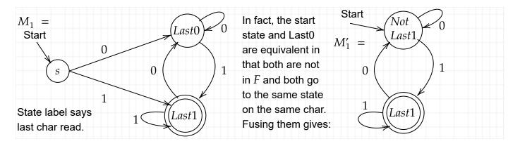
By popular demand, the table for  $M_1: M_1 = (Q, \Sigma, \delta, s, F)$  where  $Q = \{s, Last0, Last1\}$ ,  $\Sigma = \{0, 1\}$ , the start state is literally called  $s, F = \{Last1\}$ , and  $\delta: Q \times \Sigma \rightarrow Q$  is defined by
