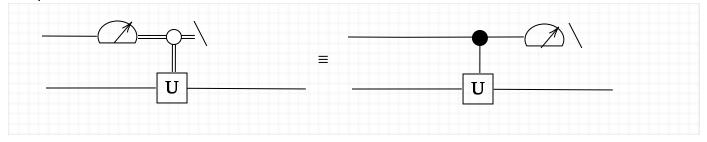
What this does is legitimize the policy of having measurements only at the end of a circuit.
