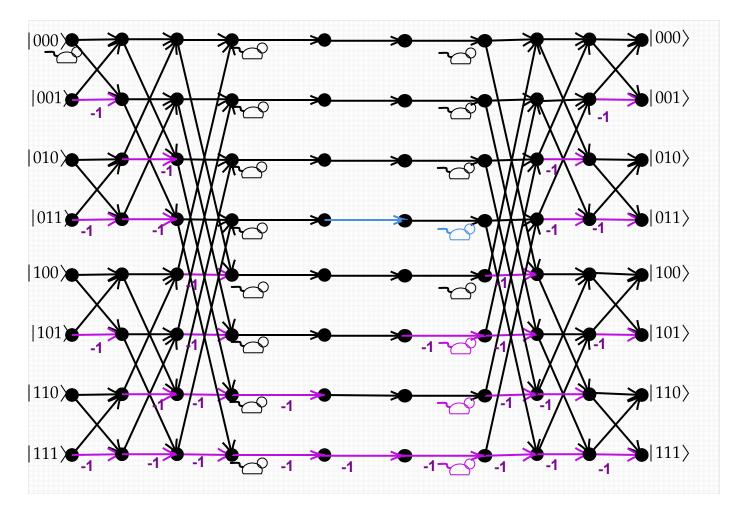
The only change was in the middle column, removing the -1 from the row for  $|011\rangle$ . The middle column now "fires" only when all 3 bits are 1, i.e., for the component of  $|111\rangle$  in any state. This is the action of the double-controlled Z-gate, CCZ (which is really a triple control of a  $180^\circ$  phase shift). It is easy to diagram in a quantum circuit:
