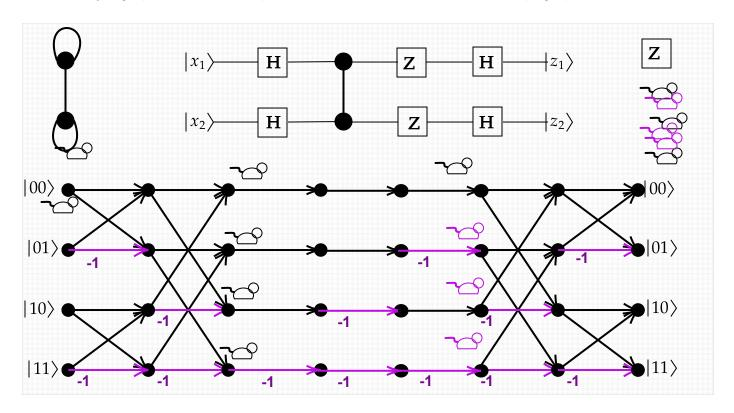
The -1 phase shifts for the **Z** gates go on the basis states that have a 1 on line 1 or 2, respectively. Now the amplitude value  $\langle 00 | U_G | 00 \rangle$  is negative. Its sign does not affect the probability and the state still gives an equal superposition.
