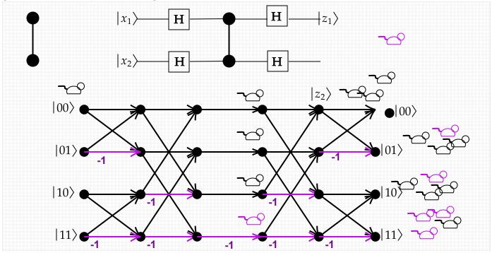
If we take the two Hadamard gates away from line 1, then we have  $\mathbf{H} \ 2 \ \mathbf{CZ} \ 1 \ 2 \ \mathbf{H} \ 2$ , which is equivalent to  $\mathbf{CNOT}$ . But with them, we get equal superpositions once again. Most in particular, the amplitude of  $\langle 00 | U_G | 11 \rangle$  (=  $\langle 11 | U_G | 00 \rangle$ ) is nonzero. [The lecture also noted how  $\frac{1}{2}[1,1,1,-1]^T$  is a fixed point of  $\mathbf{H}^{\otimes 2}$ , ignoring multiplication by the unit scalar -1.]
