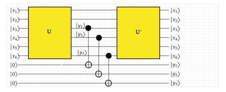
Note: this works only when it really is true that the selected lines have separated basis state values at that juncture. An example where it fails is with n=1 and r=1, the circuit  ${\tt H}$   ${\tt 1}$   ${\tt CNOT}$   ${\tt 1}$   ${\tt 2}$   ${\tt H}$   ${\tt 1}$  which creates the operation we called E.
