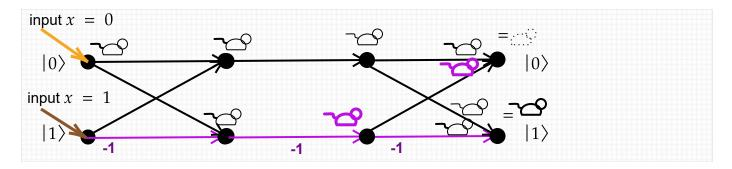
This time, when "Phil" starts running from  $|0\rangle$  at left, the "mice" cancel at  $z=|0\rangle$  and amplify at  $z=|1\rangle$ . And on input  $x=|1\rangle$  they output the basis state  $|0\rangle$ . The result is Boolean NOT, i.e., **X**.
