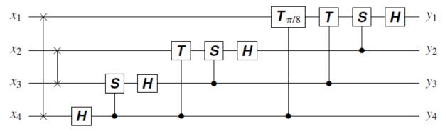
Here  $T_{\pi/8} = \begin{bmatrix} 1 & 0 \\ 0 & \omega' \end{bmatrix}$  with  $\omega' = e^{i\pi/8}$  not  $\omega = e^{i\pi/4}$  as with the *T*-gate. So  $\omega'$  has a phase angle one-sixteenth of a circle. For n = 5 the next bank uses 1/32, then 1/64, and soon the angles would be physically impossible so the gates could never be engineered.
