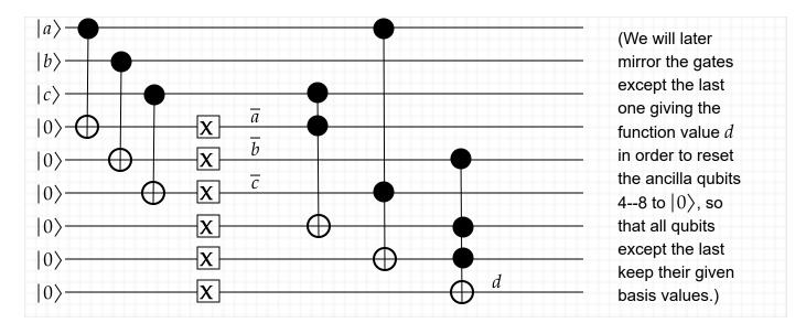
Note also that the initial three **CNOT** gates effectively copy the Boolean values *a*, *b*, *c* so that they can be negated as  $\overline{a}$ ,  $\overline{b}$ ,  $\overline{c}$  on the next three qubit lines. This is covered in section 6.2, and the last three qubit lines exemplify the trick in section 6.1 of using **NOT** gates to effectively initialize them to  $|1\rangle$  rather than  $|0\rangle$ . *Caveat:* You can't copy an arbitrary quantum state using **CNOT**---the **No-Cloning**
