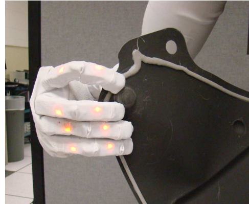
Fig. 1. Robonaut 2 hand localizing a bump in a piece of flexible plastic.
