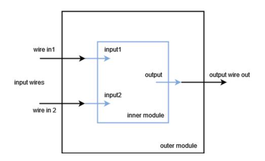
Instantiating another module inside a module by connecting their interfaces with wires.
