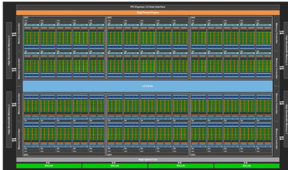
**Figure 4.15 Full-chip block diagram of the Pascal P100 GPU.** It has 56 multithreaded SIMD Processors, each with an L1 cache and local memory, 32 L2 units, and a memory-bus width of 4096 data wires. (It has 60 blocks, with four spares to improve yield.) The P100 has 4 HBM2 ports supporting up to 16 GB of capacity. It contains 15.4 billion transistors.
