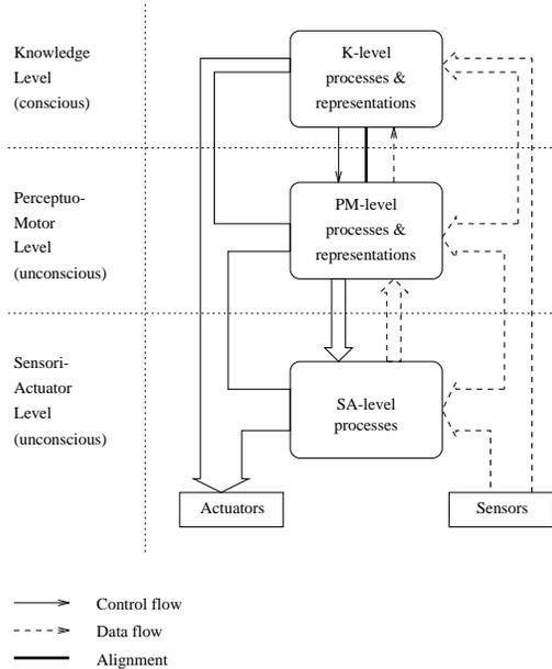
Figure 1: Schematic representation of the GLAIR architecture. Width of control and data paths suggests the amount of information passing through (bandwidth). Sensors include both world-sensors and proprio-sensors.
