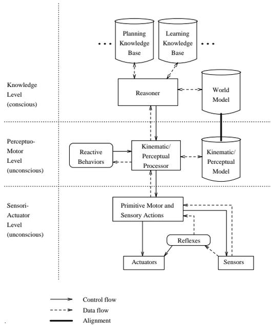
Figure 2: Schematic representation of the structure of a prototypical GLAIR-agent, an agent conforming to the GLAIR architecture.
