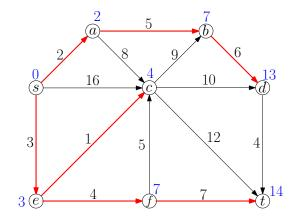
Single Source Shortest Paths Input: directed graph G = (V, E),  $s \in V$   $w : E \to \mathbb{R}_{\geq 0}$ Output:  $\pi(v), v \in V \setminus s$ : the parent of v $d(v), v \in V \setminus s$ : the length of shortest path from s to v
