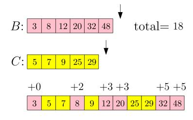
$\bullet$  Procedure that merges B and C and counts inversions between B and C at the same time
