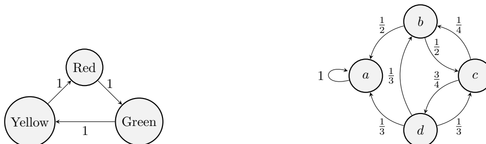
(a) Traffic light system. The traffic light can change from red to green, green to yellow and yellow to red. Each transition edge has weight 1, indicating that the transitions among states are deterministic.
