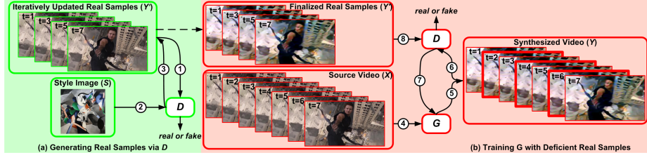
Fig. 3. Pipeline. Our method first uses a MDAN model D to generate real samples every other frame within an iterative deconvolutional process. \mathcal{Y}' is initialized with the downsampled source video \mathcal{X}' . The generated real samples are used to train G using a GAN model. Then, G transfers the image style to the whole video. The numbers on the arrows indicate the order of operations, which are explained in detail in § 3.
