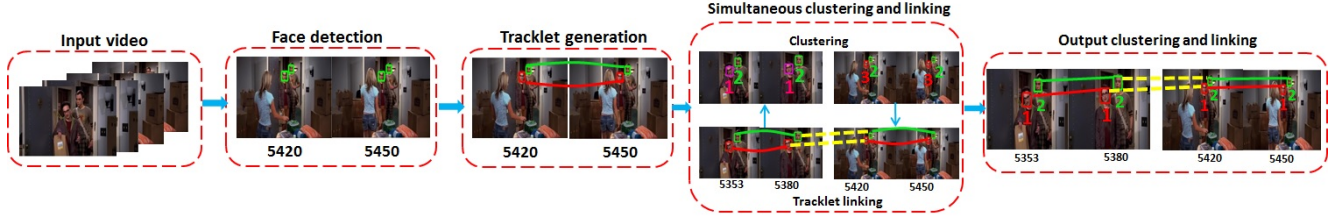
Figure 2. Overall workflow of our method for simultaneous face clustering and tracklet linking. With an input video, we first detect all faces in each frame, and then form face tracklets from adjacent frames. The face tracklets are iteratively clustered and linked into longer tracks in a bootstrapping manner, with the final output of the algorithm being the complete long tracks of detected faces with cluster labels.
