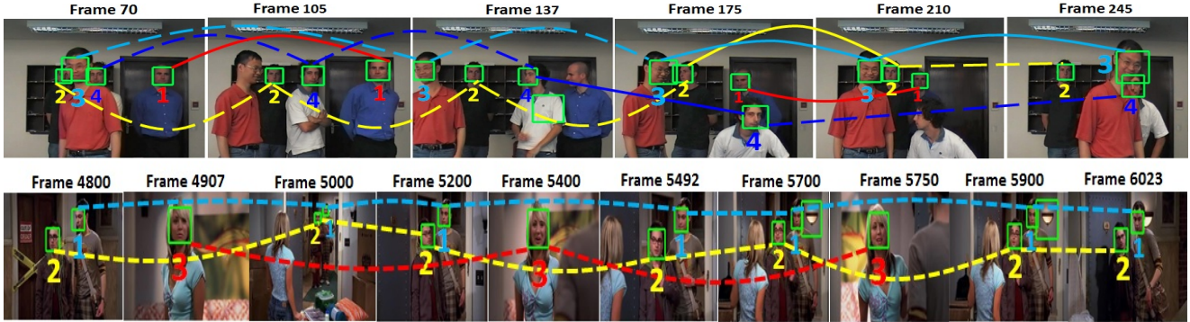
Figure 5. Illustration of the output face clustering and tracklet linking from our method on (Top) Turning and (Bottom) BBT01. The colored numbers indicate the different cluster labels. The solid curves connect detected faces of the same tracklet. The dashed curves represent linking of tracklets.
