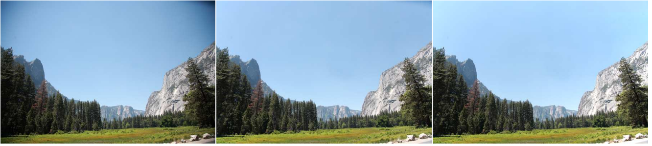
Figure 5: Vignetting correction results for images with physical vignetting. Left: a vignettted image captured with a Canon EOS 50D camera. (Courtesy of Canon USA, Inc.) Middle: image with vignetting corrected using Canon’s Peripheral Illumination Correction tool. Right: vignetting corrected with our method.
