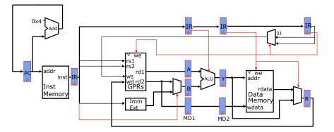
Also suppose that you have executed the following sequence of instructions with the above datapath, where "ADD R1, R2, R3" adds two registers R2 and R3 and stores the result to R1 (i.e., R1  $\leftarrow$  R2 + R3), and "SUB R1, R2, R3" substracts R3 from R2 and stores the result to R1 (i.e., R1  $\leftarrow$  R2 – R3).
