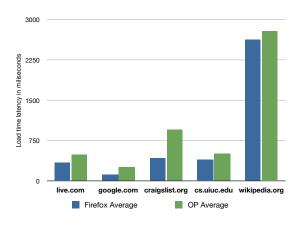
Fig. 11. Loading latencies for OP and Firefox.
