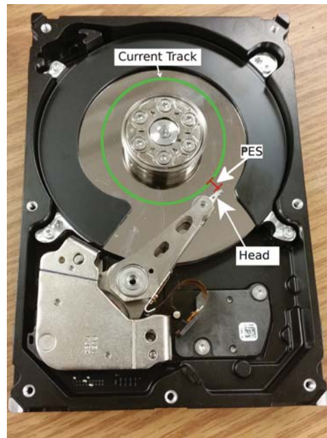
Figure 1: The Position Error Signal (PES) measures the offset of the read/write head from the center of the track.
