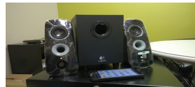
Fig. 1: Experiment setup depicting loudspeaker and the smartphone with embedded motion sensors placed on same surface .
