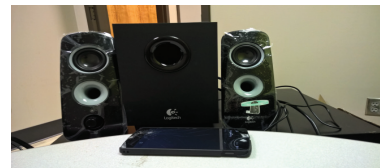
Fig. 2: Experiment setup depicting loudspeaker and the smartphone with embedded motion sensors placed on different surfaces .
