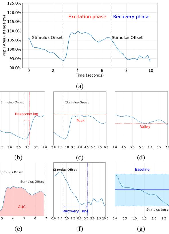
Fig. 4: (a) Illustration of excitation and recovery phase. (b) Response lag. (c) Peak magnitudes. (d) Valley magnitudes. (e) AUC (Area under the curve). (f) Recovery time. (g) Baseline.
