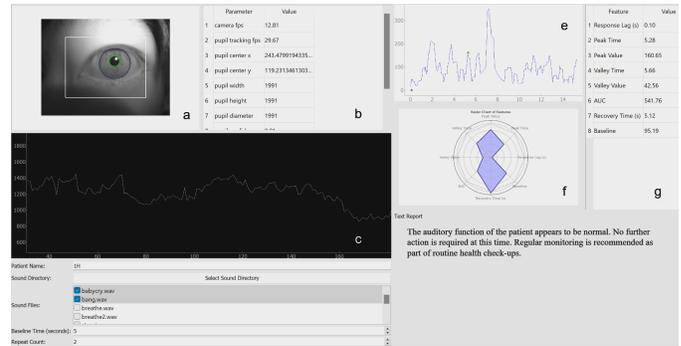
Fig. 3: UI (a) Real-time Pupil Tracking Image; (b) Parameter List; (c) Real-time Data Graph (d) Test Settings and Controls; (e) Feature Graphs for a Single Trial; (f) Radar Chart; (g) Feature Table; (h) Text Report.
