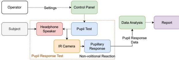
Fig. 1: The hearing disorder assessment system diagram
