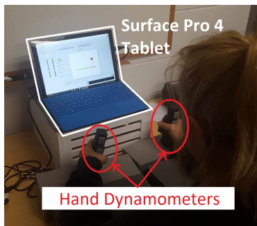
Fig. 2. System setup for an experiment with a stroke patient. The Microsoft Surface Pro 4 is employed for interface display and monitor in this trial.
