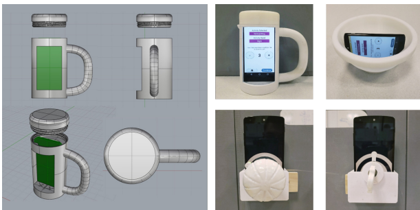
Figure 3: Left Figure: 3D visualization of the Mug in four different views. Smartphone is placed at the center to ensure the balance. Right Figure: Software-defined objects in use.
