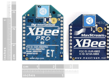
Figure 1. Dimensions of XBee Pro and XBee wireless modules.
