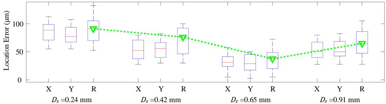
**Figure 11: Overall accuracy results: X indicates the error in the horizontal direction, Y is the error in vertical direction and R is the error along the radial direction. The parameter  $D_s$  indicates the size of droplets.**
