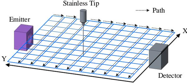
**Figure 8: Sensor calibration of light beam field using stainless tip simulation.**
