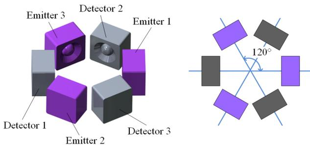
Figure 6: The sensor layout model in LuBan system.
