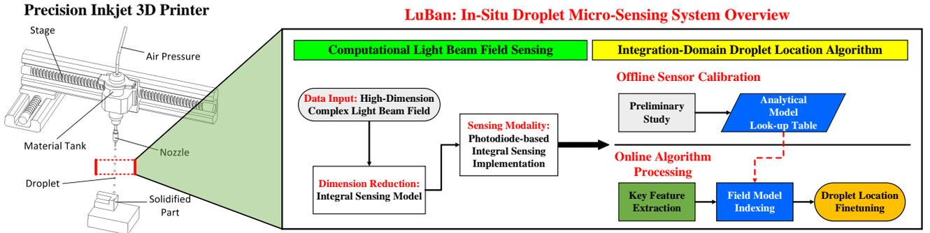
Figure 4: The system overview of *in-situ* droplet micro-sensing for inkjet 3D printing quality assurance.
