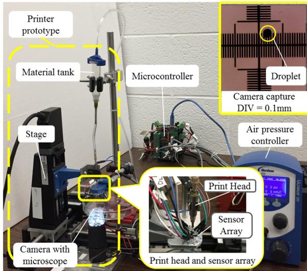
Figure 14: Prototype of our LuBan system, including 3D printer, sensor array, print head and control board.
