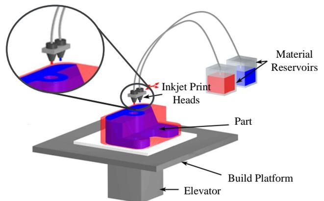
Figure 1: The inkjet 3D printer structure.
