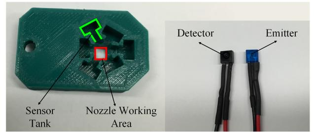
Figure 7: The working area of the printing head and sensor deployment of three pairs.
