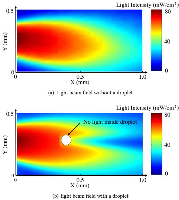
**Figure 3: An example of light beam field with and without interference from the droplet.**
