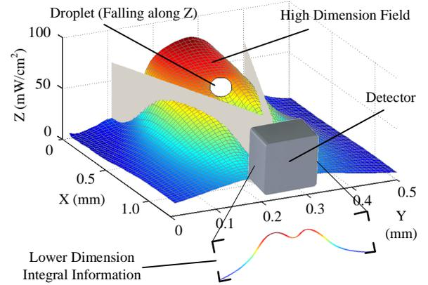
Figure 5: An example of complex field interference pattern sensing by an integral model.
