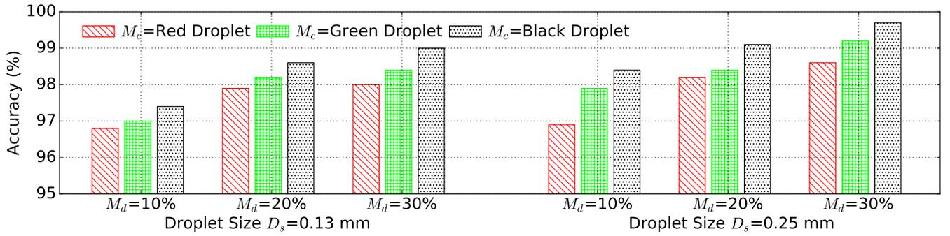
Figure 15: Accuracy of real world study. It compares the effect of droplet size ( $D_s$ ), material color ( $M_c$ ) and density ( $M_d$ ).
