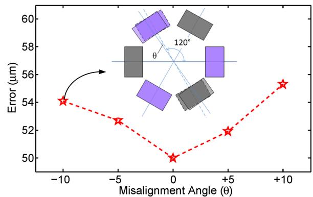
Figure 13: Accuracy under five misalignment cases. An example is provided to illustrate the misalignment.
