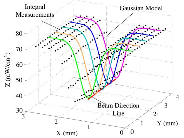
**Figure 9: Analytic model fitting for integration domain measurements.**
