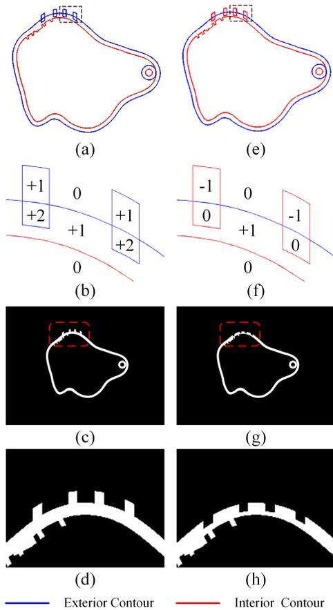
Fig. 14. Hearing Aid with Monogram: (a) contour with feature add-on, (b) winding number for feature add-on, (c) image for feature add-on, (d) zoom-in image for feature add-on; (e) contour with feature removal, (f) winding number for feature removal, (g) image for feature removal, (h) zoom-in image for feature removal.
