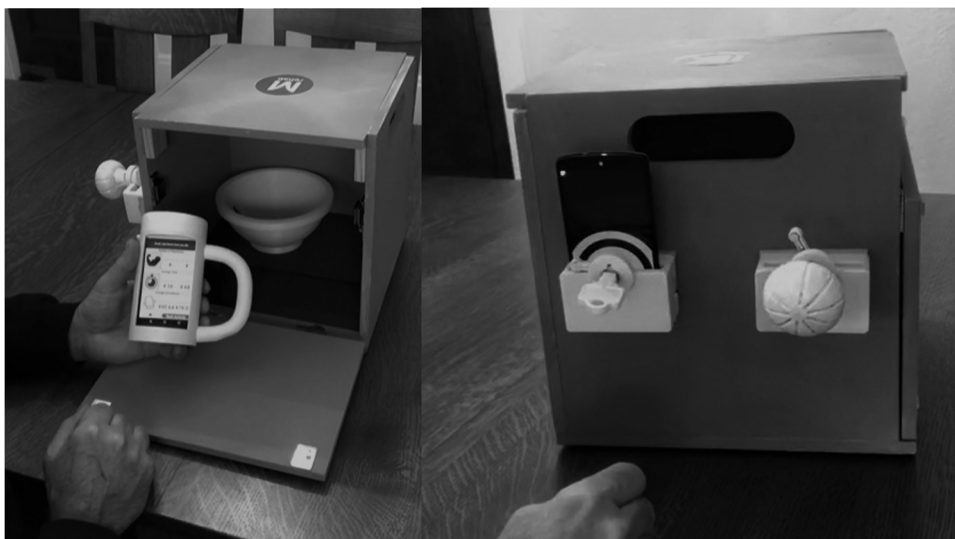
Figure 1. mRehab system including 3D printed mug, bowl, key, doorknob and box.
