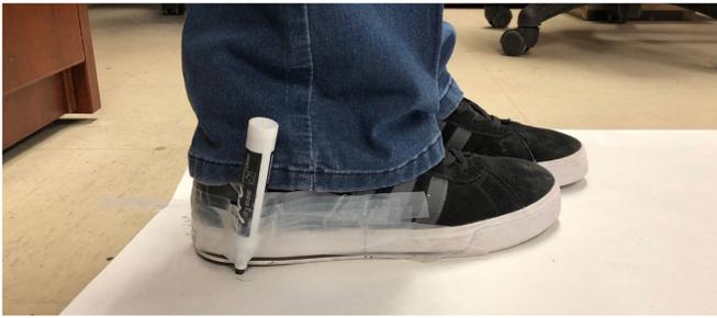
Fig. 7. Experiment setup of data labeling via the color pen at the side of each shoe. The SL ground truths are manually measured via tape measurement.
