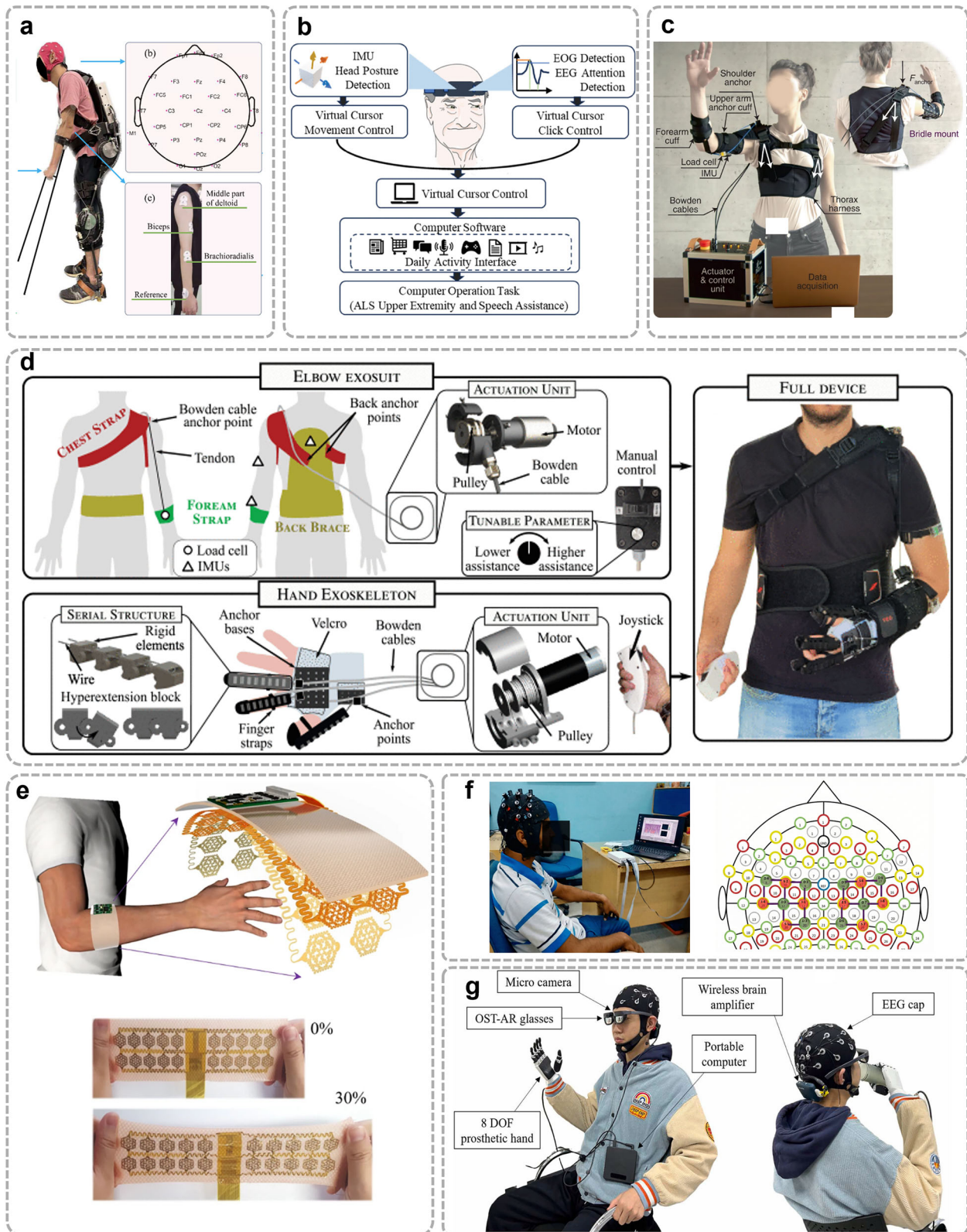
Fig. 3 | Illustration of wearable sensing technologies. a Overview of a lower limb exoskeleton using TFDP, a time-frequency method based on differential pattern analysis for feature extraction 64 . Reused with permission from Li et al. 64 . b Wearable BCI mouse system with headband, electrode placement, and schematic control framework 66 . c Textile-based exomuscle (Myoshirt) for shoulder support using tendon-driven actuation anchored on the thorax and upper arm 62 . Reused with permission from Geogarakis et al. 62 . d Soft upper-limb wearable robots including
