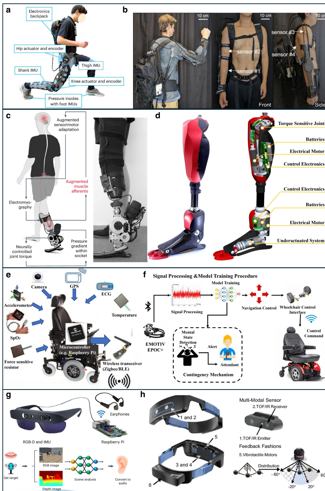
Fig. 4 | Representative implementations of wearable technologies enabling assisted mobility across different modalities. a Exoskeleton using joint moment estimation for task-agnostic support 89 , b Upper-limb exoskeleton with soft bioelectronics 45 , c EMG-driven leg prosthesis for biomimetic gait restoration 107 , d A lightweight robotic leg prosthesis replicating the biomechanics of the knee, ankle,
