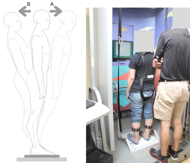
Fig. 6. Left: A Demonstration of displacing COG from center to front and from center to back. Right: Equipment set up. The test subject is wearing Wearable Gait Lab while standing on dynamic force plate of the Smart Balance Master system.
