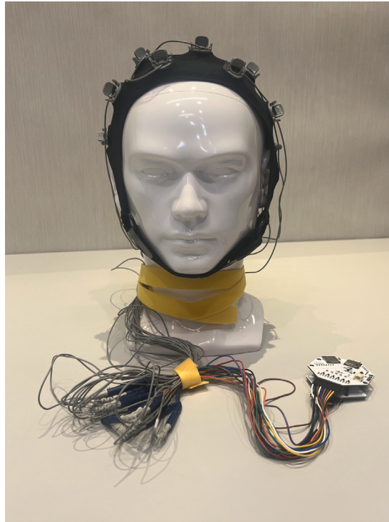
Fig. 3. EEG sensor system: A wearable head cap equipped with multiple electrodes for capturing brain activity signals.
