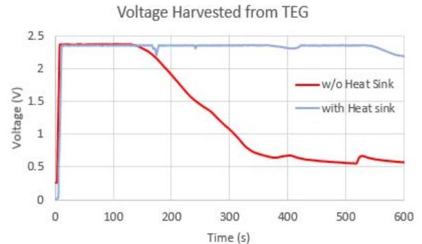
Fig. 2. Voltage harvested using *LTC3108* without load connected. Note that the user movement caused the voltage to decline at end of reading with heat sink.
