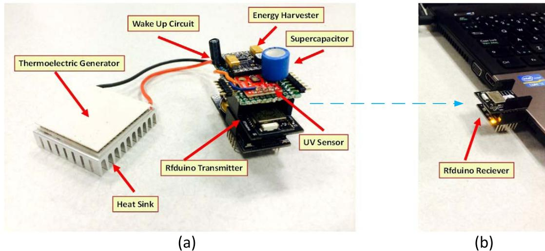
Fig. 6. Personalized ultraviolet exposure monitoring system prototype, (a) Main system including TEG, heat sink, wake up circuit, supercapacitor, energy harvester, UV sensor, and RFduino transceiver. (b) RFduino receiver connected to a computer to collect data.
