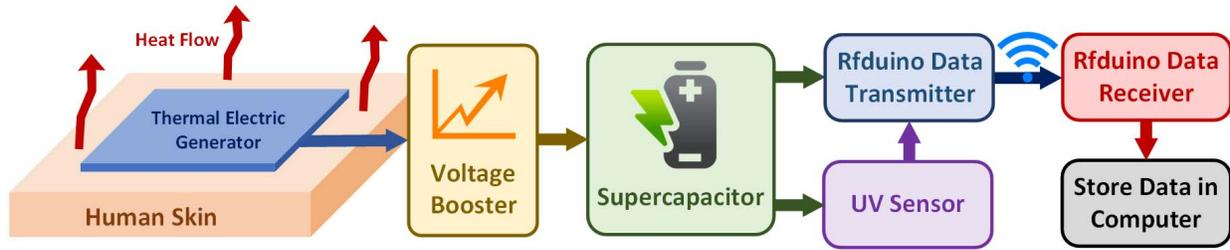
Fig. 1. The system architecture and data flow of the self-powered system. Energy is harvested by TEG from human skin and stored in the supercapacitor, which later will be used for powering UV sensor and RFduino transmitter.
