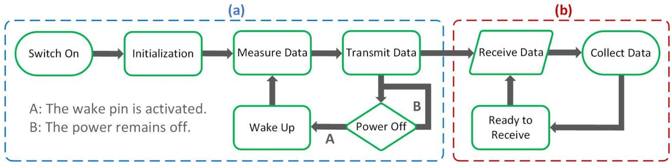
Fig. 4. The overview of the software control diagram for the RFduino data transmitter and receiver. First the user must turn on the device manually, then the RFduino initializes the RFduino Gazelle (GZLL) protocol via Bluetooth and connects to the host of RFduino data receiver.
