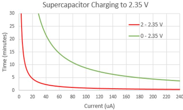
Fig. 3. Charging the 22 mF Supercapacitor from 0 to 2.35V versus 2 to 2.35V. Charging from 0 to 2.35V takes much more time than from 2 to 2.35V.
