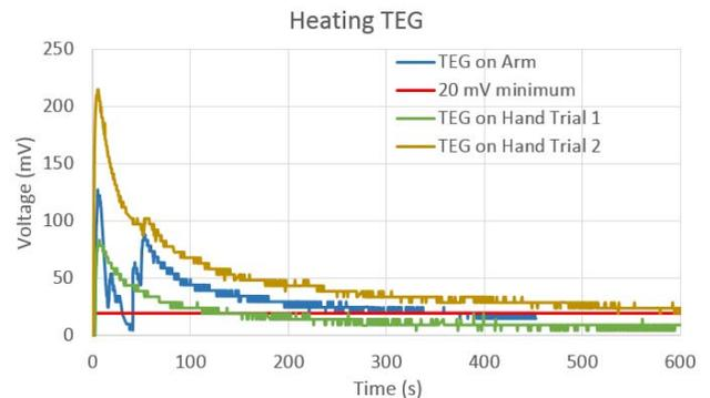
Fig. 7. TEG voltage output after applied heat with arm and hands. The measurement from arm starts at around 50s because of the initial noise from movement. The voltage obtained from hands is higher than the one obtained from the arm.
