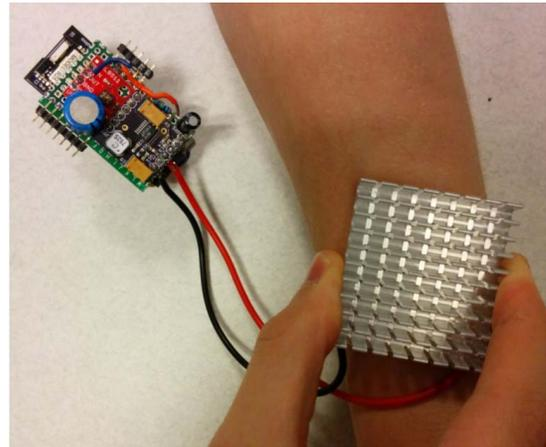
Fig. 5. Heating TEG on the arm. The other side of the TEG is cooled by the ambient air through the heat sink.
