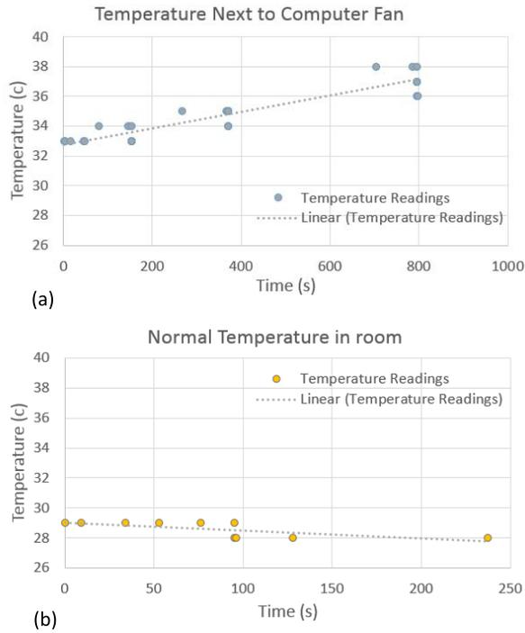
Fig. 8. Temperature data collected in the second experiment. (a) Temperature increase linearly versus time when the temperature sensor is located near a computer fan. After about 800s, the temperature increases about 5 degrees. (b) Temperature decrease a little versus time when the sensor is located in an office room.
