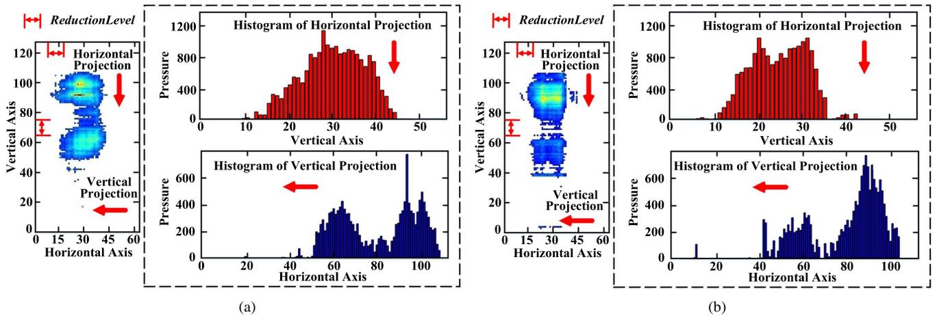
Fig. 10. Horizontal and vertical histograms with projection descriptor of (a) left fetus and (b) supine ( $\text{ReductionLevel} = 3$ ). The pressure image are projected to horizontal and vertical directions, and the pressure image is described with histograms in a line. It should be noted that the number of grids in the pressure image is much less than the number to produce the projection histograms in both (a) and (b), which is for clear explanation.
