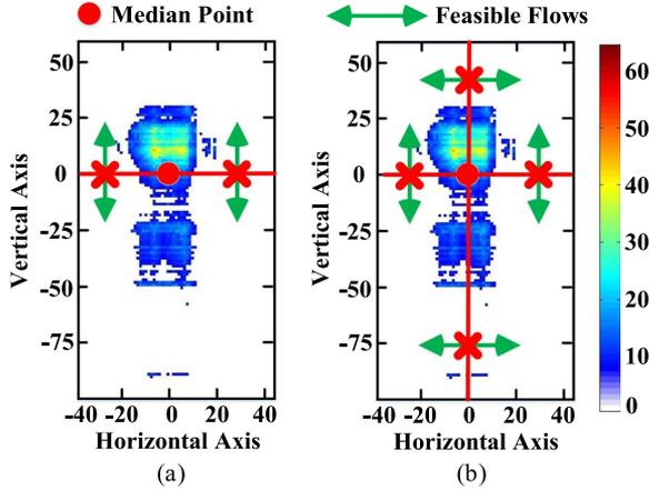
Fig. 12. Two region segmentations with median point as the segmenting point. (a) Upper-lower segmentation. (b) 4-region segmentation. By segmentation, the feasible flows between the segmented regions are cancelled.
