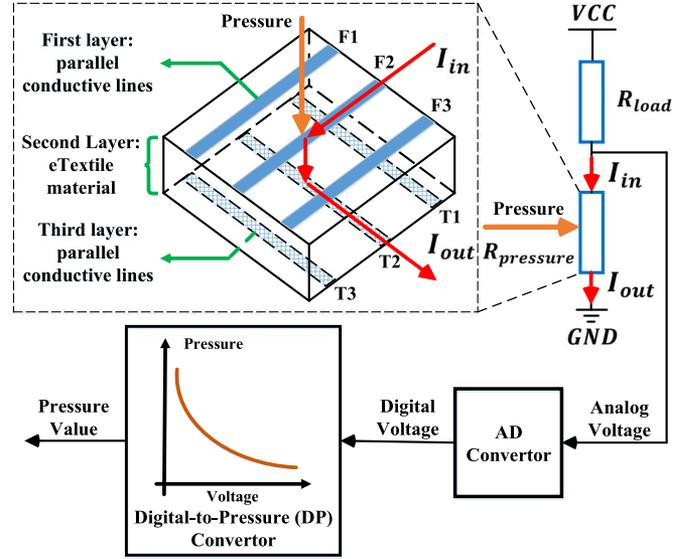
Fig. 4. Illustrations of the Smart Bedsheet system with a  $3 \times 3$  pressure sensor array: each of the first and third layer has three conductive lines and are orthogonal. The middle layer contains eTextile material, which is pressure-sensitive.
