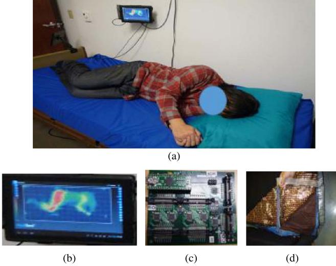
Fig. 3. (a) The Smart Bedsheet system in use and its submodules. (b) Terminal (a tablet). (c) Scanning module. (d) E-textile with conductive lines.
