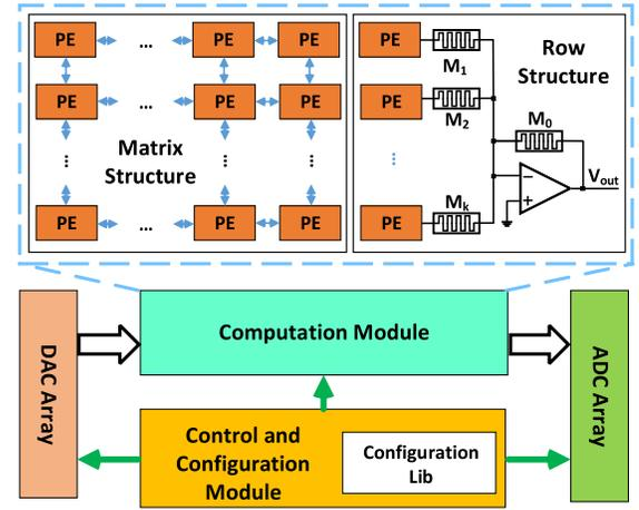
Fig. 1. Architecture of the distance accelerator, MDA.
