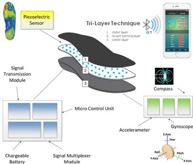
Fig. 1. System architecture of Smart Insole, which includes an array of sensors and a GUI.
