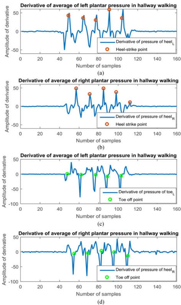
Fig. 9. Derivative of plantar pressure from both feet. (a) Left heel strike. (b) Right heel strike. (c) Left toe-off. (d) Right toe-off.
