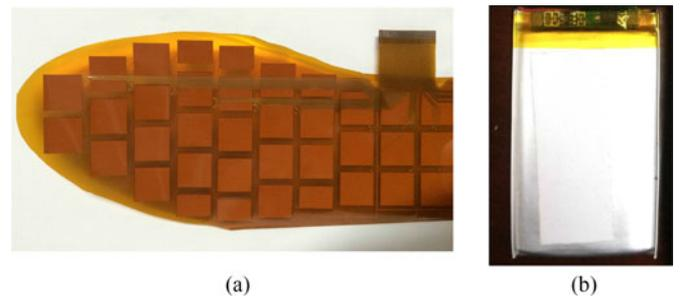
Fig. 3. Pressure sensor array and rechargeable battery of Smart Insole (a) The pressure sensor array and circuit connection (b) The rechargeable battery.
