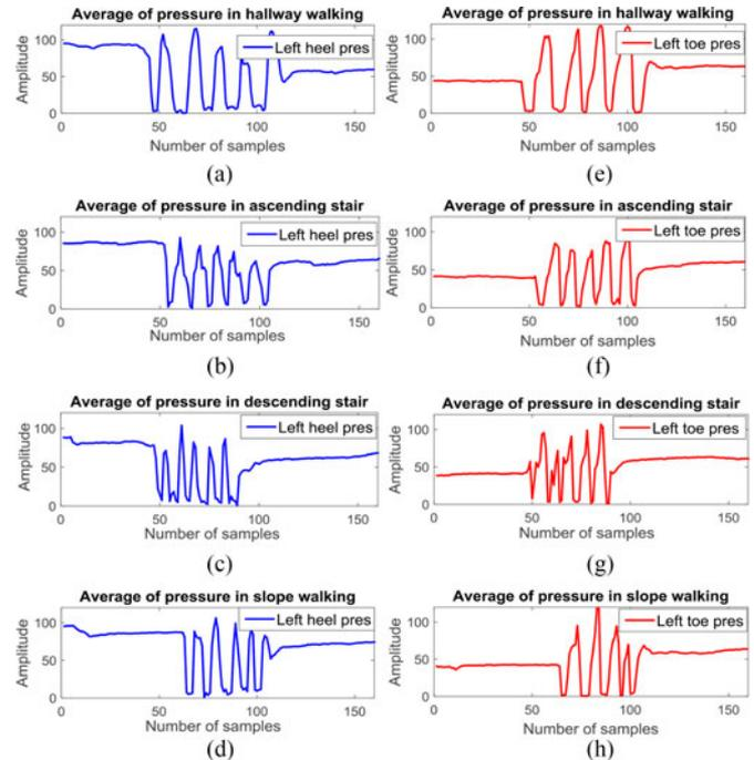
Fig. 8. Left plantar pressure from both heel and toe groups in different scenes. (a) Heel pressure in hallway walking. (b) Heel pressure in ascending stairs. (c) Heel pressure in descending stairs. (d) Heel pressure in slope walking. (e) Toe pressure in hallway walking. (f) Toe pressure in ascending stairs. (g) Toe pressure in descending stairs. (h) Toe pressure in slope walking.
