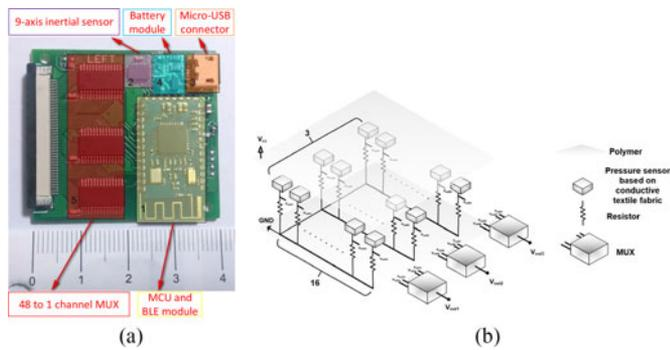
Fig. 2. PCB and pressure sensor array circuit of Smart Insole (a) The PCB design (b) The diagram of pressure sensor array circuit.
