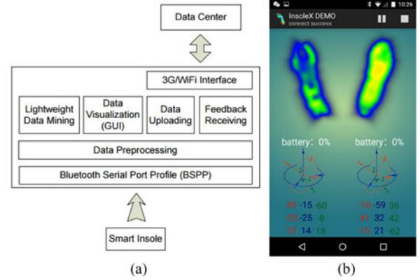
Fig. 5. Software of Smart Insole. (a) Stacked software structure. (b) Data visualization GUI on a smartphone software.
