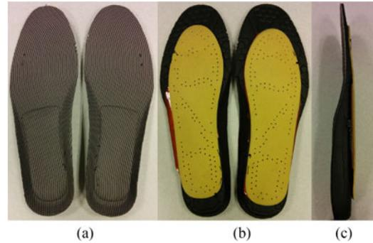
Fig. 4. Human ergonomic prototype of Smart Insole. (a) Front view. (b) Back view. (c) Lateral view.
