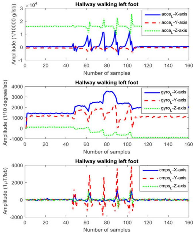
Fig. 11. IMU data from left foot in a hallway walking, from top to bottom are accelerometer, gyroscope, and magnetometer data.
