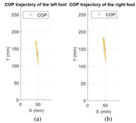
Fig. 10. Trajectories of COP shifting in hallway walking. (a) Left foot. (b) Right foot.
